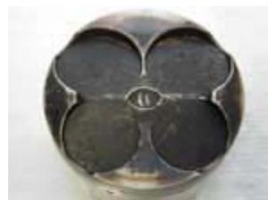
The curved squish areas are on the left and right raised sides of this piston. The flat squish areas are on the top and bottom in this picture.
