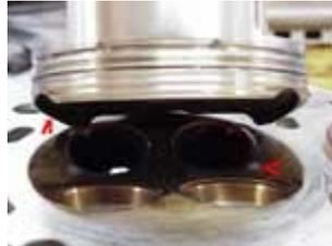
Here you can see **how** the fuel/air mixture is forced to the center of the chamber.
