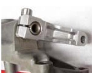
Super light clutch actuator and magnesium cover !
