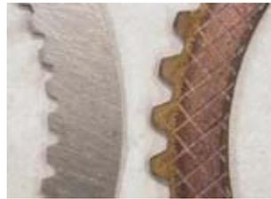
When a streetbike wet clutch is slipped hard during a race start, a lot of friction plate debris gets into the engine oil.
