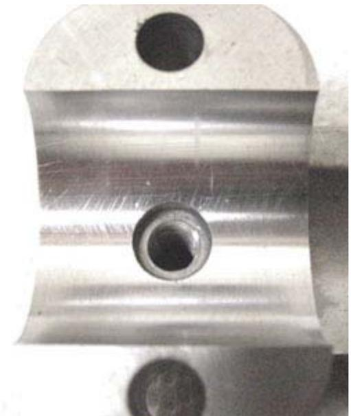
This Yamaha R6 cam cap has gone 10,000 racing miles with no metal to metal contact !!
