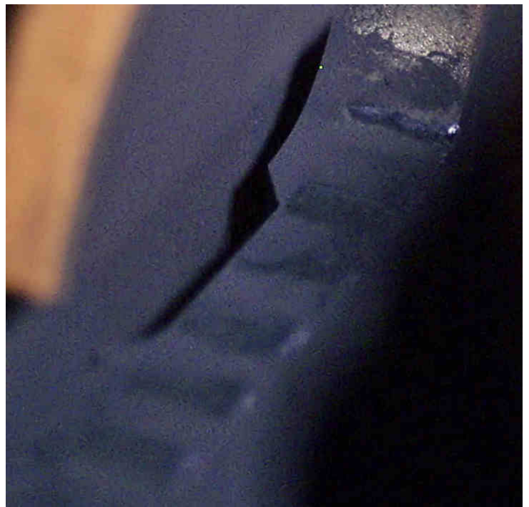
Basket Condition, note dent in bottom of slot (top of pic) where original square end dug in compared to the scrubbing marks of the “temporary” angled version a little higher up.
