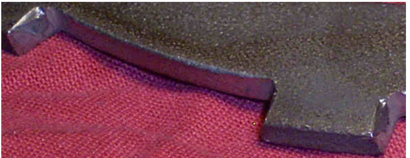
Paso Plate After 30,000km on "temporary" mod, note slight burring has started
