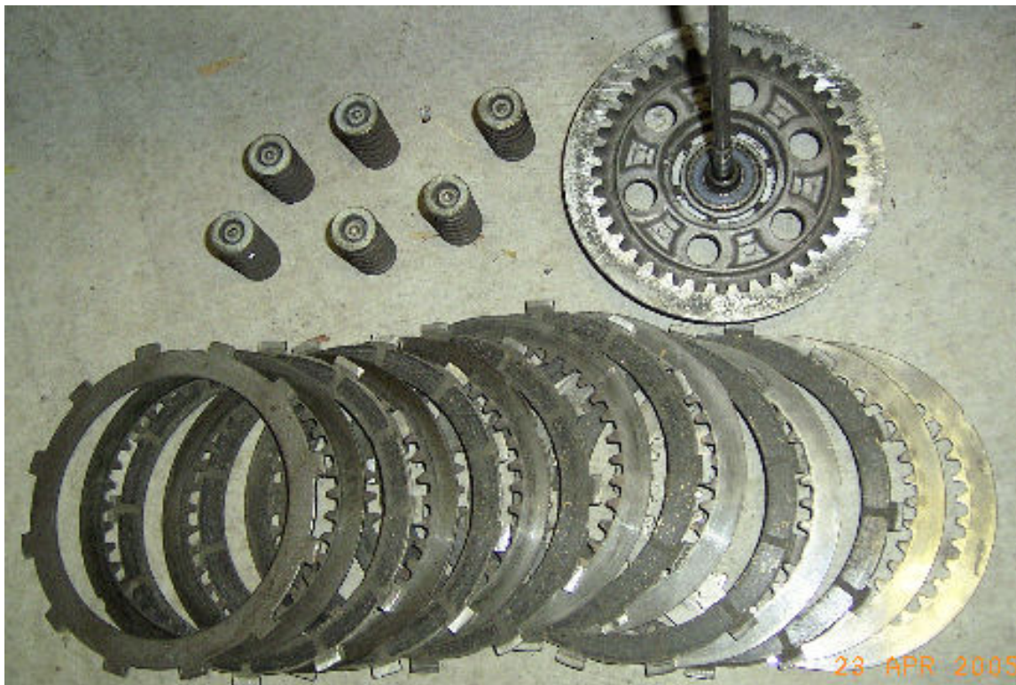
Clutch Plates, ST4S – 2003, Paso plate is on top of the pile. Note burrs removed from pressure plate
